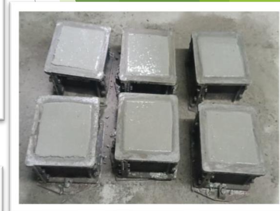
Concrete Cube Casting
