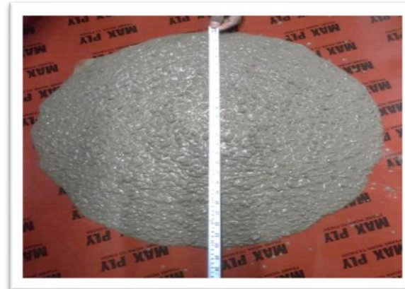
Concrete Flow Test
