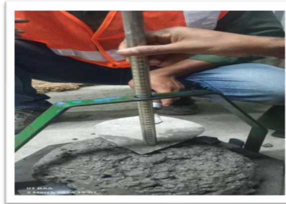
Slump Cone Test
